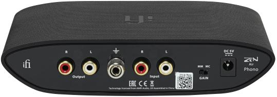
At rear, gold plated phono input and output terminals, an earth pillar and small MM/MC slide switch. This actuates internal switching to change both gain and load, logic circuits managing the change over to prevent thumps.
