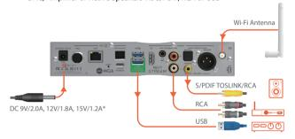
\*A power supply unit must be able to deliver minimum rated repetitive current.
