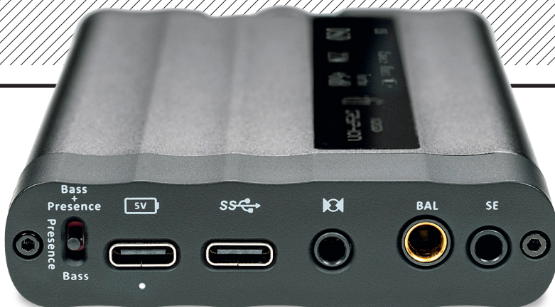
ABOVE: The xDSD Gryphon provides single-ended (3.5mm) and balanced (4.4mm) sockets that act as inputs in analogue headphone amp mode and as line outs in DAC/preamp mode. One 3.5mm S/PDIF and two USB-C inputs serve digital in and battery charging, respectively, with bass/presence response shaping toggled nearby
