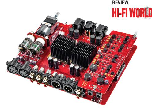
It may look like a computer motherboard, but this complex but orderly construction actually lives within the Pro iCAN Signature's distinctive enclosure. We can also see the output stage heatsinks, motorised ALPS volume control and two horizontallymounted 'new old stock' GEmade 5670 miniature double-triodes.
