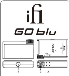
1. Power on/off, Bluetooth format annunciation, Voice alert on/off and digital filter mode on/off Power switch
