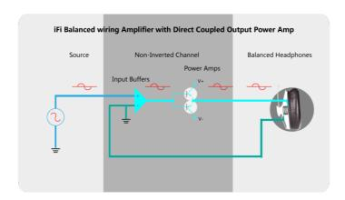
With S-Balanced, a dedicated negative wire per channel all the way to the starground of each channel's amplifier to ensure there is no crosstalk between the channels.
