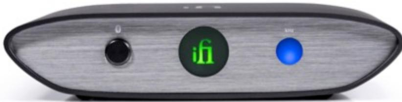
The LED at the centre of the ZEN Blue's front panel changes colour to identify the Bluetooth codec being received, while another LED to the right indicates the sample rate. Qualcomm's QCC5100 chip can be updated over-the-air, enabling future Bluetooth codecs to be added to the ZEN Blue's specification.
