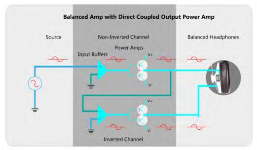
In the Balanced amp topology, the second amplifier doubles both signal levels versus an unbalanced amplifier, which makes this good for power-hungry, less sensitive headphones. A dedicated negative wire per channel makes sure there is no crosstalk between them, which is a plus for regular balanced outputs, but headphones/IEMs finished with TRS jacks are not compatible. This is where the hipdac also has S-Balanced which makes iFi portable components unique.
