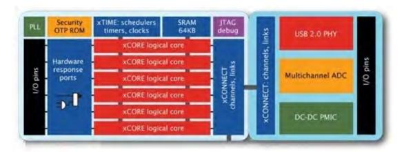
The hip-dac implements Version 4 AMR XMOS platform and uses the latest generation 8-Core 500MIPS XMOS1 transputer derived main processor. These processors are quite unique in their architecture and based on a technology once considered to revolutionize computing, the INMOS Transputer.
