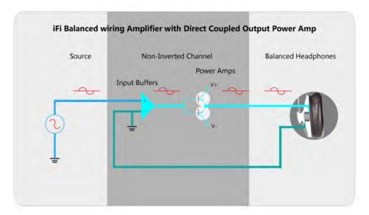
With S-Balanced, no second amplifier is used, neither are extra signal, noise, nor distortion added - perfect for sensitive IEMs. A dedicated negative wire per channel all the way to each channel's amplifier's star-ground makes sure there is no crosstalk between the channels.
