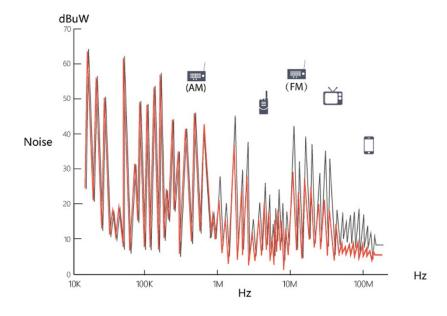
With local sources of noise, these range from linear power supplies (yes, they make noise!) to switch-mode power supplies to digital circuitry and all the related harmonics.
