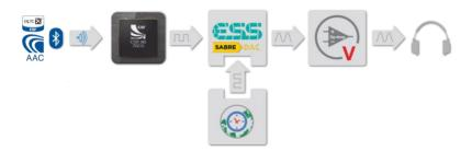
The signal from SOC has a huge amount of jitter so it is then sent to an ESS Sabre Hyperstream DAC chipset with Time Domain Jitter Elimination and discrete oscillator, to eliminate jitter for conversion to analogue, before being sent to the amplifier.
