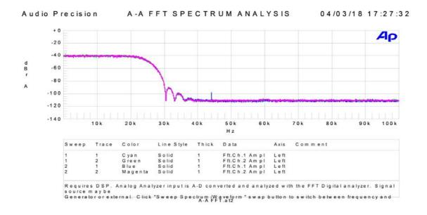
It is clearly observable that the filter response using white noise is dramatically different from any of those presented for 5.20 & 5.30. Other than the precise waveform and filter response differing if MQA processing is engaged, these results parallel those expected if MQA processing was engaged for non-MQA streams.
