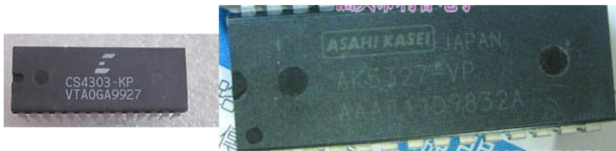
Crystal CS4303 Delta Sigma DAC and Asahi Kasei AK5327 Delta Sigma ADC
