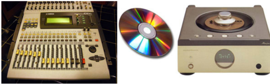
Yamaha 01V Digital Mixer with single-bit ADC's and 16 Bit PCM output to CD to Marantz CD-Player with single-bit DAC
