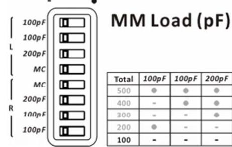
If the required load value is 100pF, all micro switches shall be in the “-”(left) position.
