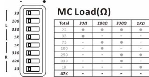
If the required load value is 47kΩ, all micro switches shall be in the “-”(left) position.
