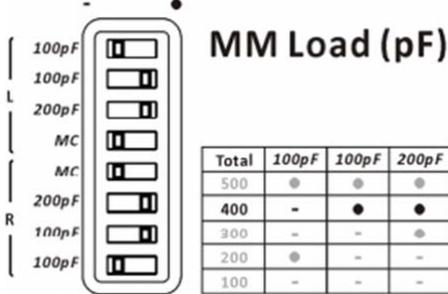
If the required load value is 400pF , then the 4 micro switches 100pF and 200pF shall be in the “●” (right) position; other micro switches shall be in the “-” (left) position.
