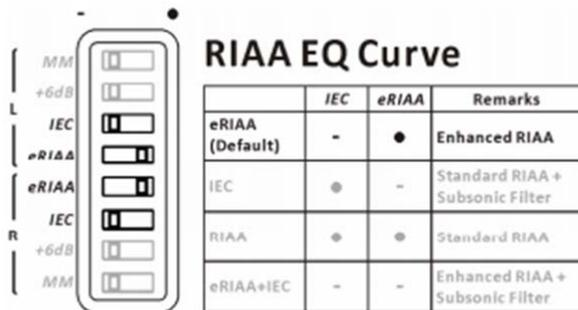
Two eRIAA micro switches should be in “●” (right) position; two IEC micro switches shall be in “-” (left) position.
