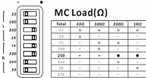
If the required load value is 250Ω, then the 4 micro switches 330 Ω and 1k Ω shall be in the “●” (right) position; other micro switches shall be in the “-” (left) position.
